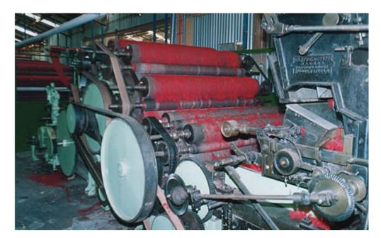
As the fibre leaves the first part of the card it pass' through heavy steel rollers, called "Peralta rollers" that are set to a very fine tolerance these rollers. The carded wool passes between the rollers, which results in vegetable matter being crushed but they do not harm the fibre. The fibre is then collected at a centre draw unit and transferred overhead to another feed table that delivers it to the second or finishing unit of the carding machine.
