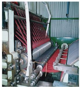
fibre to the other side and, most importantly, they rub the wool sideways, back and forth, causing the strip of wool to be rolled and condensed. It's a similar action to rubbing and rolling tobacco as an 'old timer' would to roll an cigarette. The action of rolling the fibres together give the strip of fibres some strength. Finally, the fibre strips, now called pencil roving, is wound on spools. 14 "ends" of pencil roving on each spool. The fibre is now in a form that is ready to be spun.
