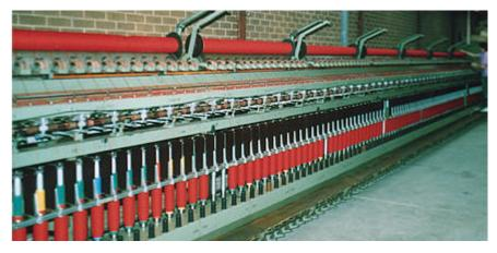
To explain how this happens, first the spools of pencil roving produced by the carding machine are placed on a drive drum at the top of the spinning frame. As the spool turns, the 14 ends from each spool are unwound into the spinning machine. The route the ends take is this - compression point, twister head, compression point and finally, the bobbin. Here is what happens. "Drafting" takes place between the two compression points. Each
