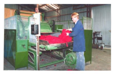
**Carding** - this is the most important process in yarn making. Carding the fibres determines the quality of the resulting yarns in terms of yarn weight, and thickness of yarn.
