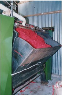
length of the machine. Additionally, the amount of fibres entering the carder is strictly controlled via a clock work scale mechanism and the distribution of the fibres is evenly placed across the width of the card, thus ensuring even, uniform pencil rovings being despatched from the machine. In all there are 84 ends of rovings simultaneously produced from the machine as it operates.
